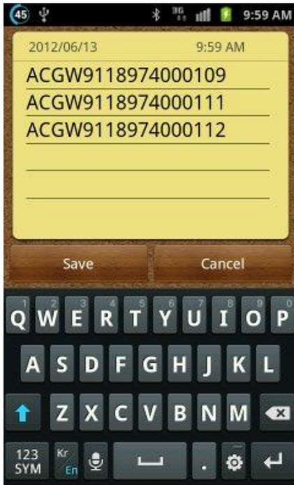
Pls. open the “Memo application” on the device and then try to scan by reading the available barcodes you need then the data will be transferred to the memo app. like this pic.
