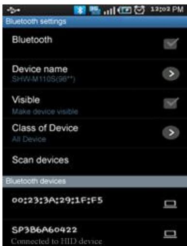
Once pairing is done, you can see the following message that “Connected to HID device”, it means HID pairing is completely done, now is ready for scan.
