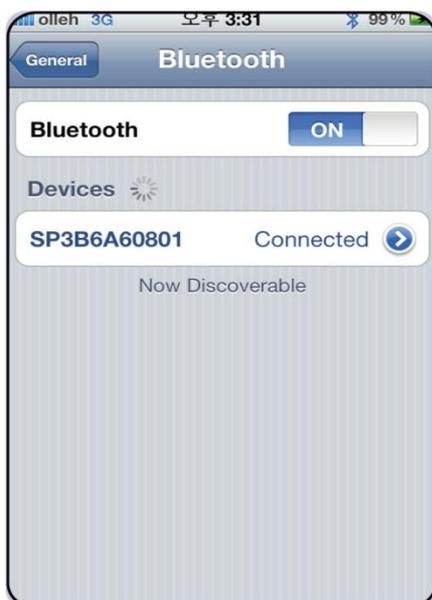
If your connection is done successfully with your device, the following message "Connected" will be shown on the screen with a beep sound, it means that the scanner's pairing is completely done.
